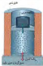
$$P_1V_1 = P_2V_2 \text{ و } \frac{\Delta V}{V} = -\frac{\Delta P}{P}$$
